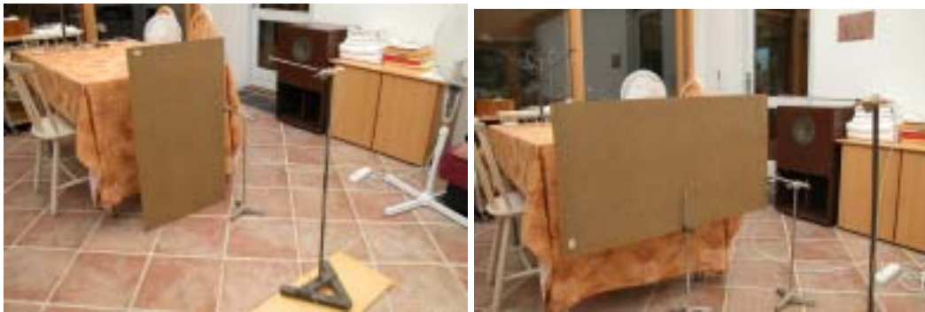
Figure 46 – Measurement set-up for the frequency response with an infinite edge using a fan as sound source. The baffle was located vertically and horizontally to test for the influence of the diffraction around the baffle ends.
