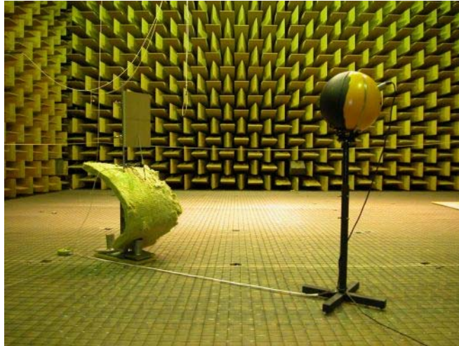
Figure 14 – The measurement set-up showing the baffle and probe microphone (left) and the source loudspeaker (right).
