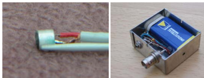
Figure 25 – The microphone was glued to a thin rod and a screened wire soldered to the terminals and battery-powering was used to reduce noise injection from mains hum.
