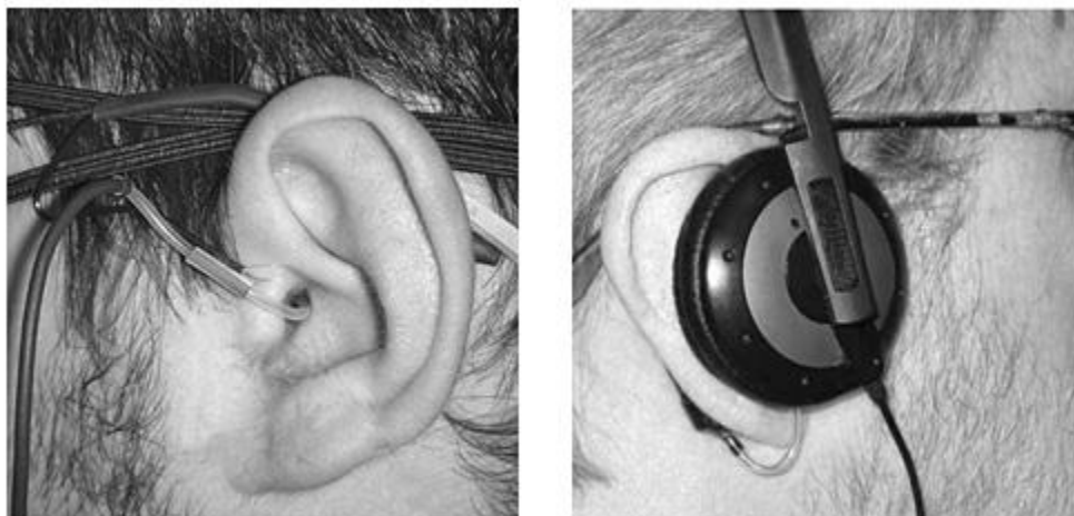
FIG. 1 Binaural recording and reproduction of the eardrum signal
