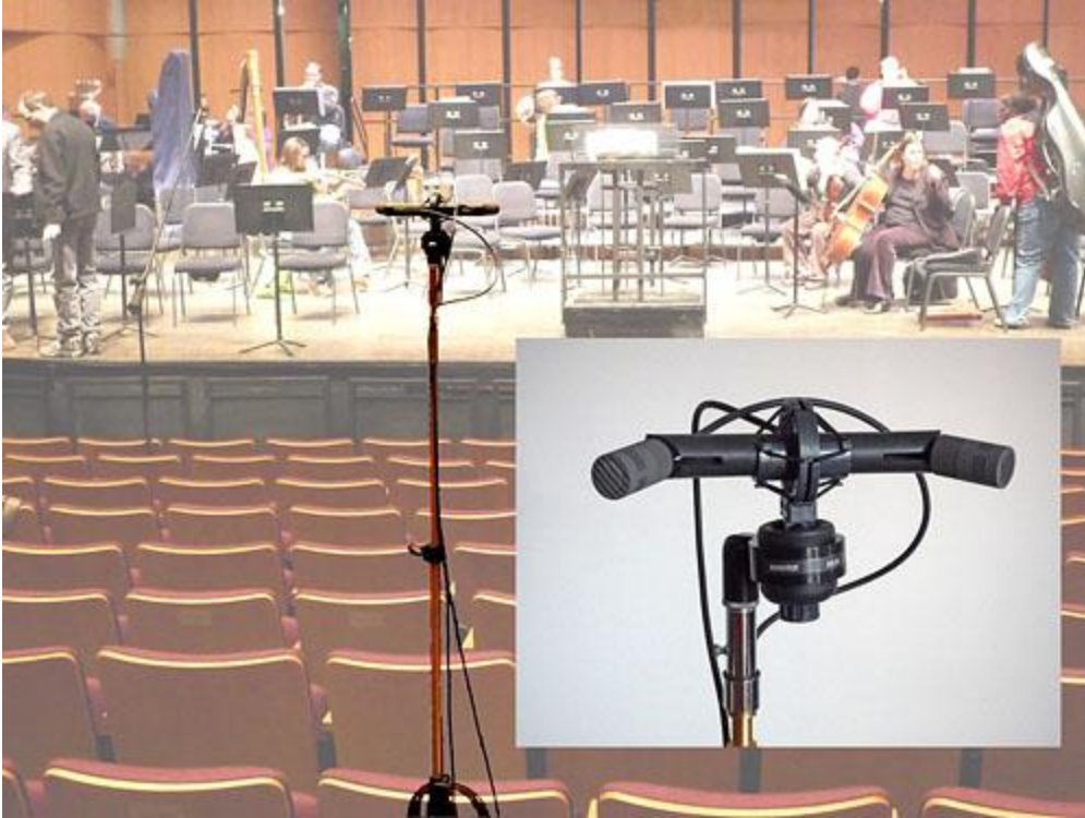
Fig. 11 Near-coincident pair of microphones. They are mounted at an angle to each other and to a stand with two shock mounts.
