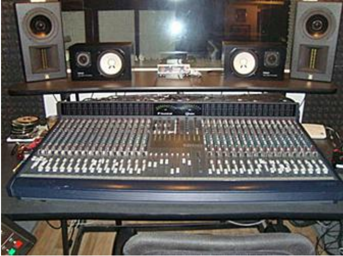
Fig. 6 32-channel mixing-board and recording monitors to create a phantom acoustic scene from up to 32 individual signals
