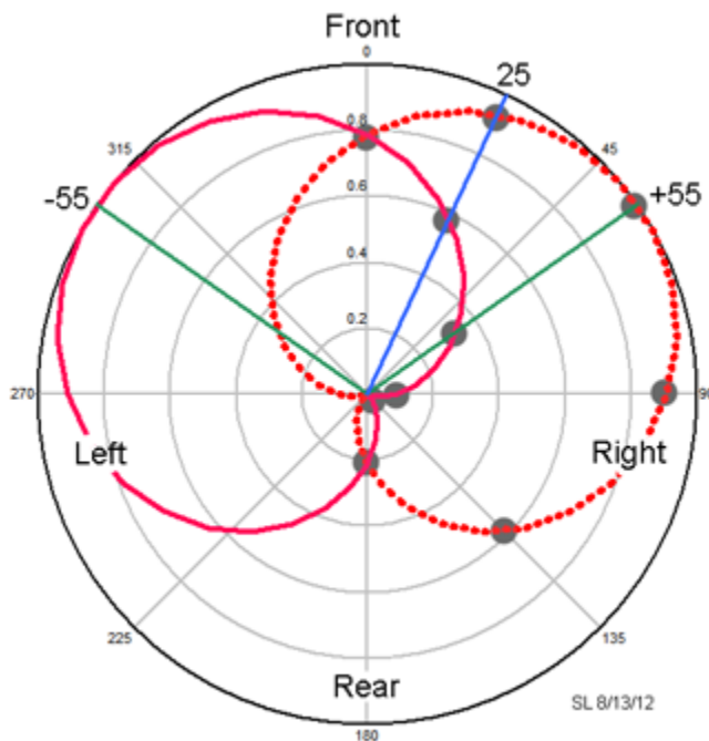
Fig. 9 Polar responses of two cardioid microphones at \pm 55^\circ angle to each other in the horizontal plane and mounted on top of each other for coincident sound arrival at the
