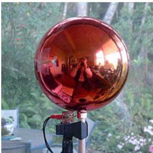
FIG. 3 Microphone capsules placed on the surface of a 19 cm sphere
