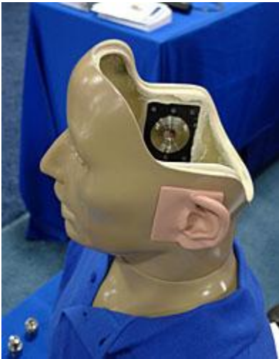
FIG. 2 Artificial head, opened to show microphone mounting fixture and outer ear
