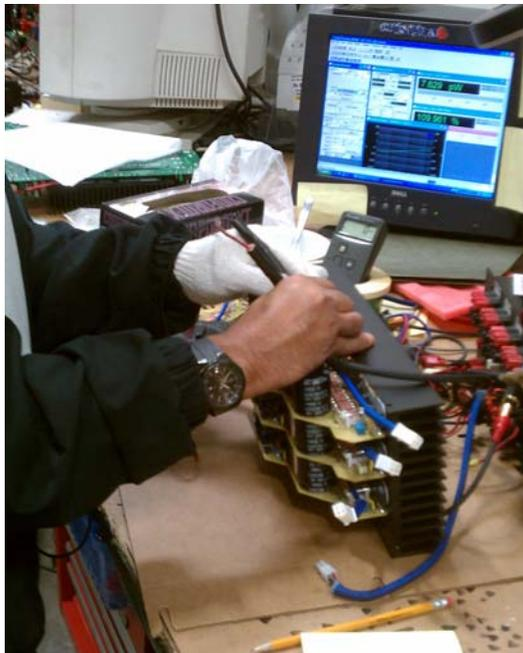
*Using our Audio Precision equipment to test amplifier modules. Modules that pass all tests are moved into the production area. Units that fail are sent to our technicians for re-work.*
