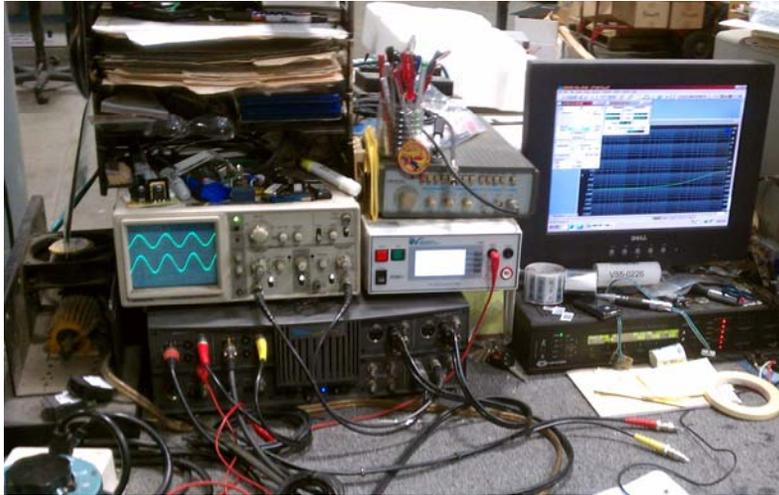
*Once everything is loaded and secured, every amplifier is hooked up to an Audio Precision test station for final testing including safety, triggers, all inputs and outputs, power output and distortion. We even short each channel at full output to verify proper operation of the protection circuitry.*
