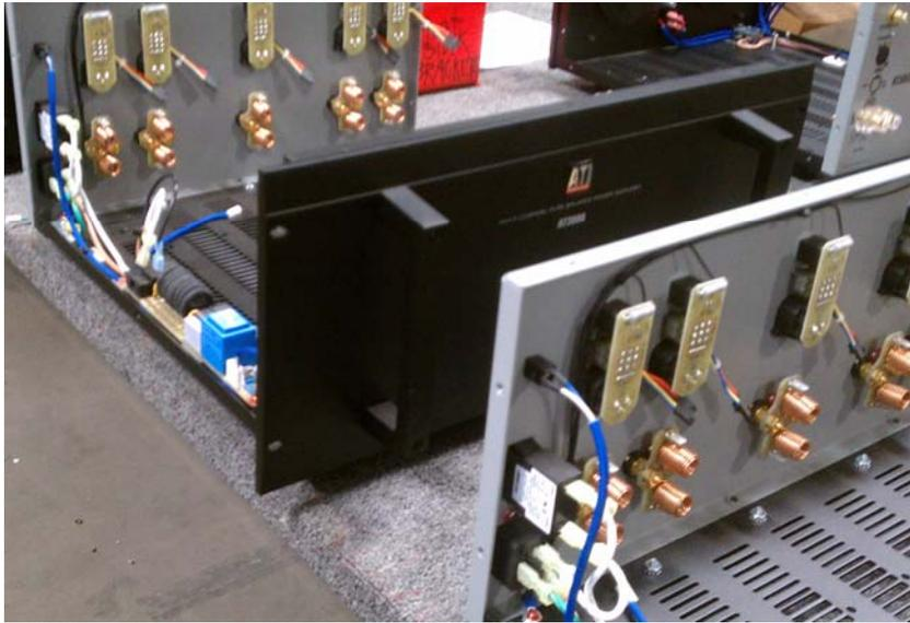
*AT3005's with rear panel connectors and Softstart modules installed.*
