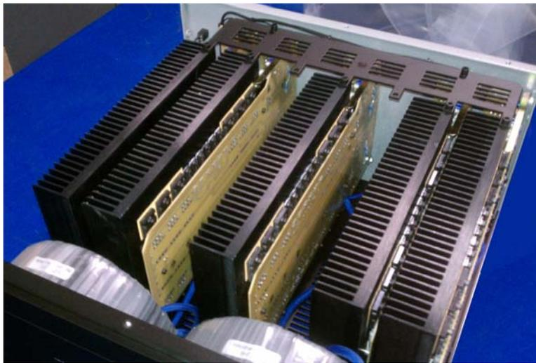
*AT3005 fully tested, loaded and waiting for the top cover. After the top cover is installed, the units are cleaned and boxed.*
