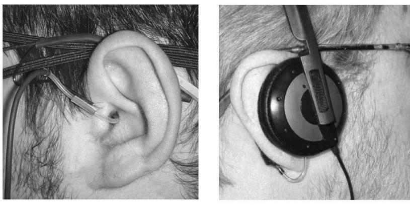
*Figure 2:* (a) Recording the sound pressure streams at the eardrums using a small diameter, flexible tube with a small microphone capsule at its remote end. (b) Headphone reproduction after the signal transmission chain has been equalized using the same tube microphone.
