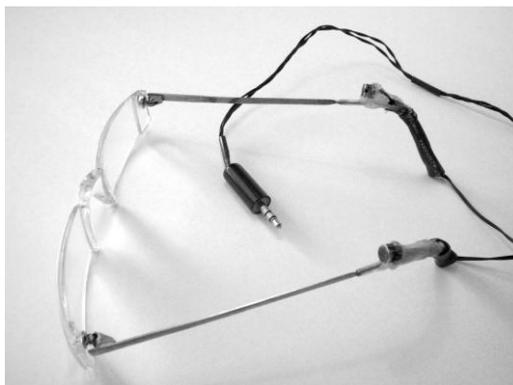
Figure 11: Recording with microphones on the sides of the head, excluding the pinna.
