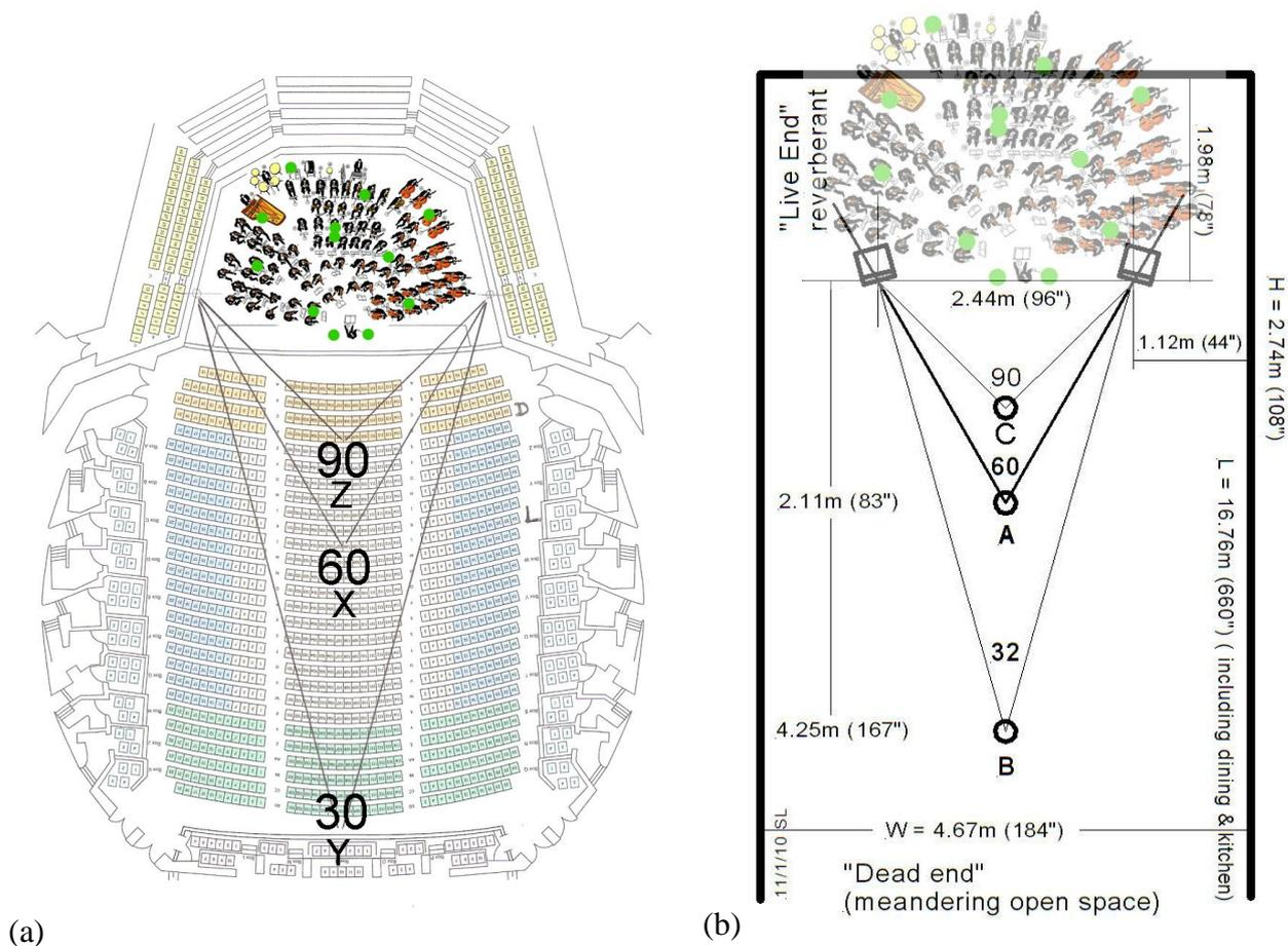
Figure 14: The  $60^{\circ}$  angle of perspective in a concert hall (a) and in a living room (b). The distances to the orchestra are about 10 times larger than to the loudspeakers.
