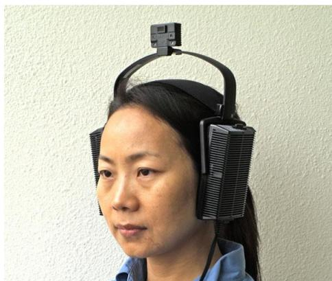
*Figure 3: Example of a motion tracker on top of the head band (Smyth Research)*
