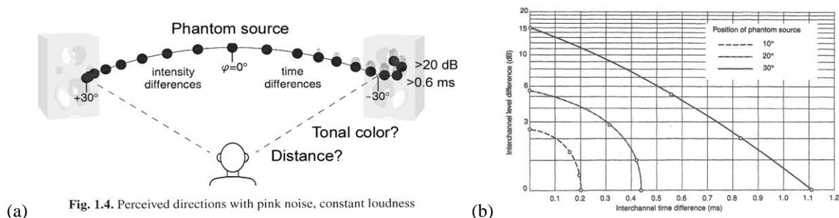
Figure 10: Amplitude or delay panning of a source to any position between two loudspeakers (a). Amplitude or time differences required to pan a source to 10°, 20° and 30° off-center (b).
