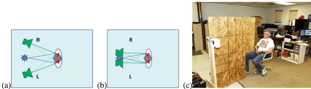
Figure 8: Crosstalk cancellation. Normal stereo setup (a). “Stereo Dipole” setup for crosstalk cancellation and a wide phantom sound stage (b). Setup with mechanical barrier, which replaces the electrical compensation of the loudspeaker drive signals (c)
