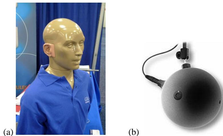
Figure 4: Artificial head (a) and sphere microphone (b)
