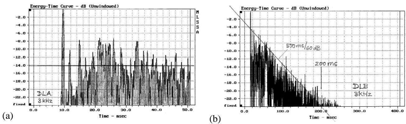
Figure 6: Direct and reflected signals for a 3 kHz toneburst from the left dipole loudspeaker in Fig.1 and Fig.14. (a) At location A during 50 ms. (b) At location B during 400 ms. [14]
