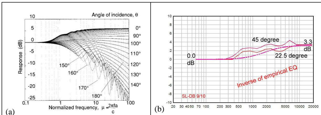
Figure 9: Sound pressure at a fixed point on a rigid sphere for different angles of sound incidence (a). Sound pressure at  $22.5^0$  and  $45^0$  incidence relative to  $0^0$  incidence for a 17.5 cm sphere (b). The dotted curve is the inverse of the loudspeaker equalization.
