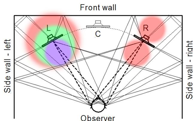
Figure 12: A typical box loudspeaker L is omni-directional at low frequencies and becomes increasingly forward directional at higher frequencies. A dipole loudspeaker R can have a frequency independent radiation pattern.
