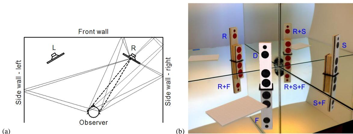
Figure 5: Direct sound and reflections from a mono loudspeaker in a room (a). Model of a dipole loudspeaker near a room corner and its reflected images (b).
