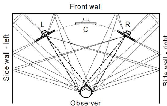
Figure 7: Monaural phantom source between two loudspeakers
