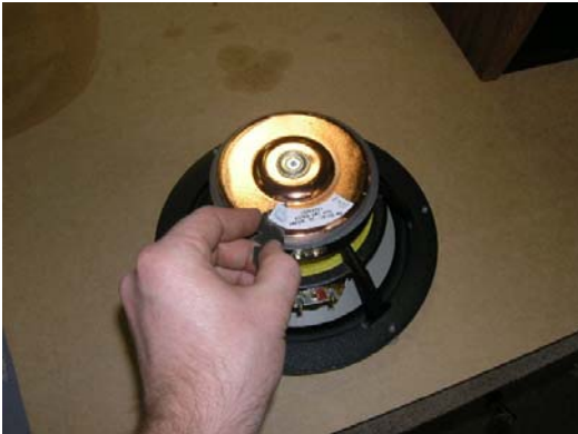
Remove the label and plastic from the driver
