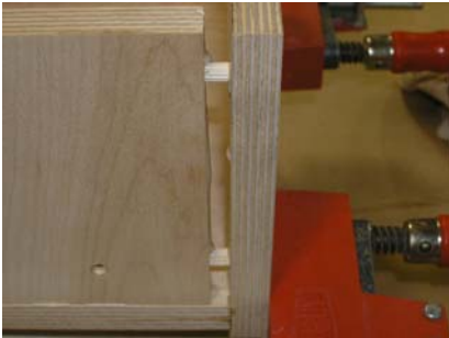
Inserting H into FT (picture showing dowels)
