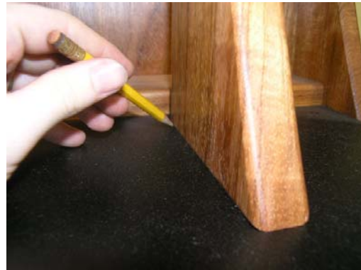
Lightly outline the foot print of the bracket onto the woofer cabinet
