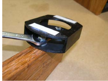
The puck and bracket assembly. (No spacer strips needed in 0.1A revision)
