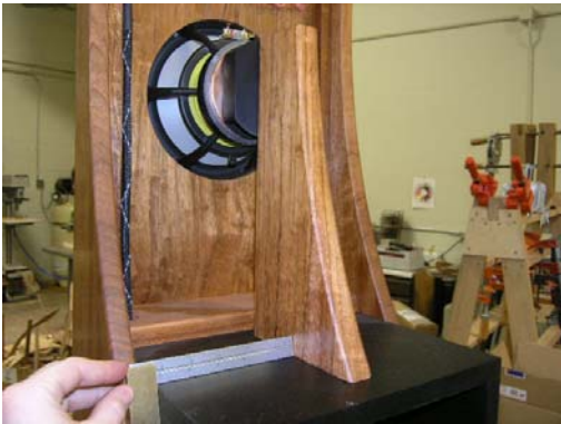
Center the puck and bracket assembly on the driver.
