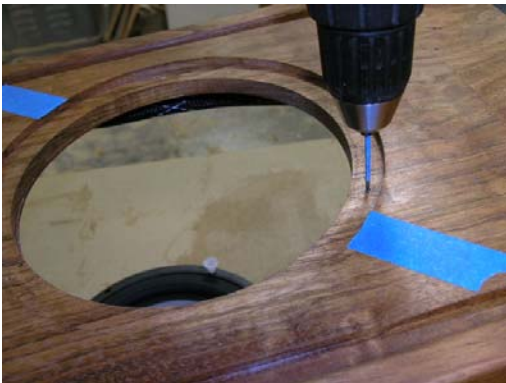
A 3/32 drill bit is shown to deepen the three mounting holes to 3/8" deep. DO NOT DRILL THROUGH THE PANEL.
