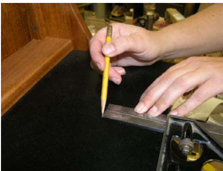
Locate the mounting holes at 2 1/2" and 4-1/2" from the back of the woofer cabinet.
