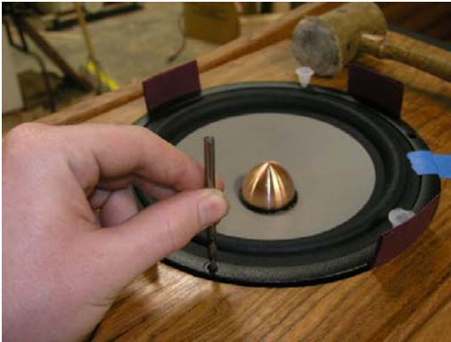
Locate the three mounting holes for the driver. A 3/16 drill bit is shown.
