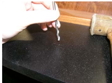
Use a center punch or the 3/16" drill bit and wooden mallet to mark the drill holes.
