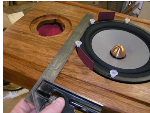
Square the driver with the electrical connection toward the top of the speaker.
