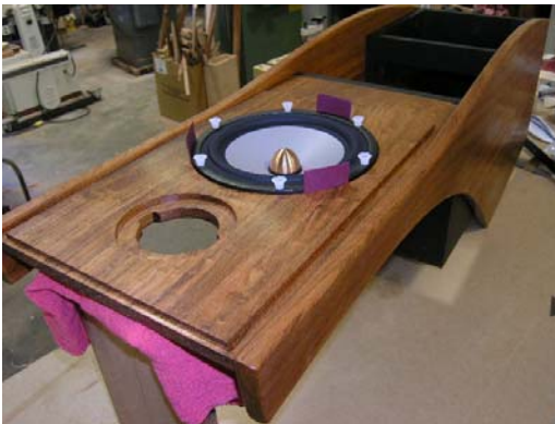
Using card stock to center the driver on the panel.
