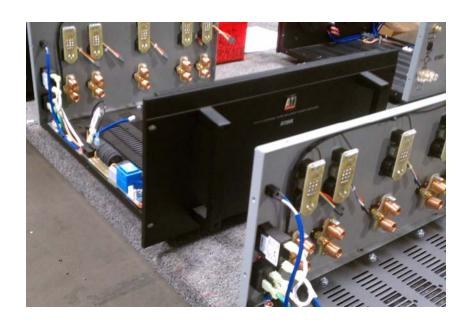
AT3005's with rear panel connectors and Softstart modules installed.
