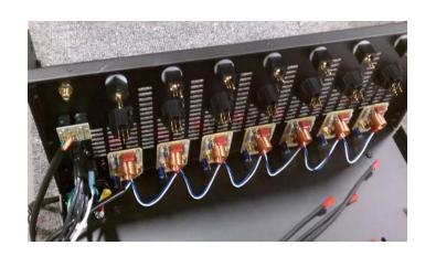
While the boards are underway, connectors are mounted directly to the chassis. This robust construction helps our legendary reliability.
