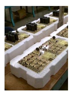
These are power supply boards on the insertion line. Once all the parts are inserted, the boards go to the wave solder machine. We use a tinonly solder so all of our units are ROHS compliant.
