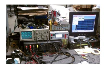
Once everything is loaded and secured, every amplifier is hooked up to an Audio Precision test station for final testing including safety, triggers, all inputs and outputs, power output and distortion. We even short each channel at full output to verify proper operation of the protection circuitry.
