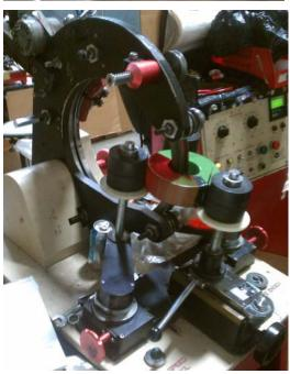
Bi-filar transformer winding machine manufacturing a multi-channel toroidal transformer.
