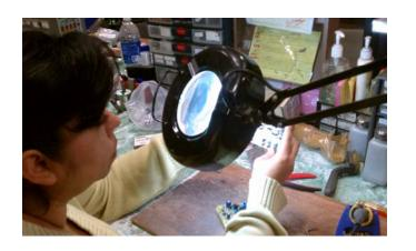
More board inspections. While it is said "you cannot inspect quality into a unit", certainly failure to inspect allows errors to pass into later production stages where they are more costly and disruptive.
