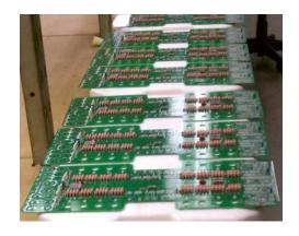
With parts and chassis on hand, boards go to the insertion line where the components are inserted by hand.
