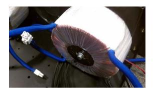
This transformer powers 4 amp channels. Note the space-age fiberglass dress on the leads and the plug-in power connectors.
