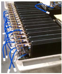
Completed and tested modules waiting to be installed in a chassis.
