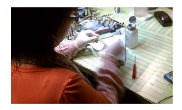
After soldering, the boards are cleaned and inspected. Any rejects are sent to be re-worked.
