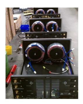
After the rear panel connectors and Softstart module are installed in the chassis, both transformers are bolted in. The next step is to install the completed and tested amplifier modules.
