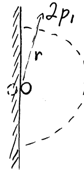
SINGLE SOURCE ON BAFFLE AND PERFECTLY SPHERICAL WAVES
