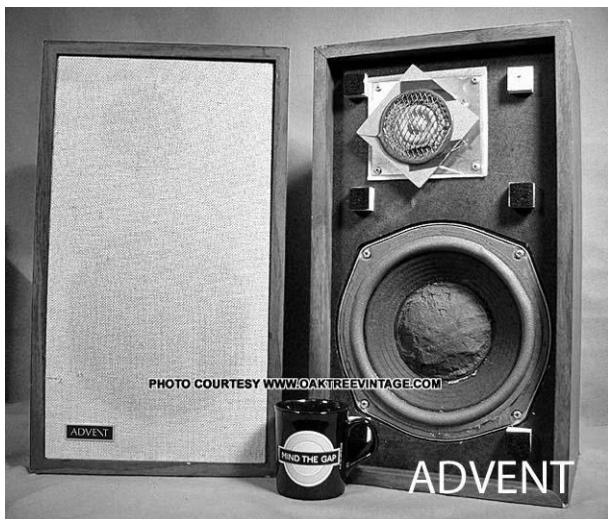
Figure 3: Small ADVENT speaker with novel tweeter.
