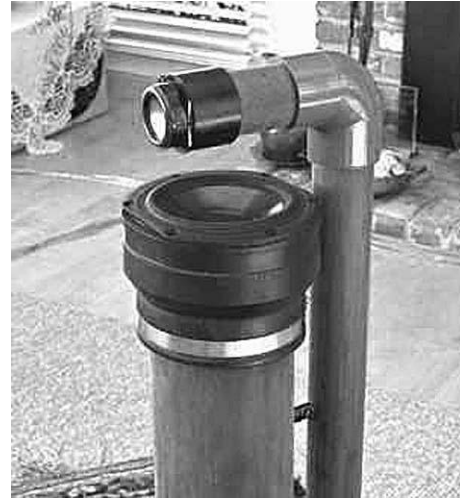
Figure 27: Wide dispersion 2-way loudspeaker
