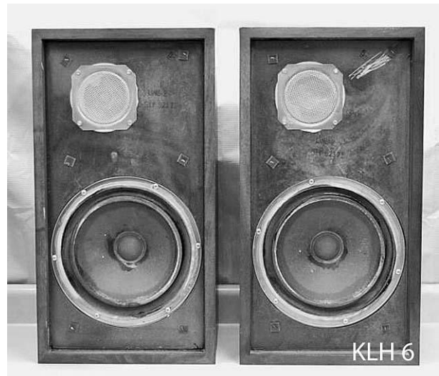
Figure 1: Two-way loudspeaker with “acoustic suspension” woofer in a sealed box.
