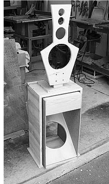
Figure 29: Open baffle construction for a full-range dipole loudspeaker [16].
