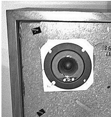
Figure 2: Tweeter with small dome and large paper surround
