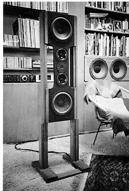
Figure 18: Open-baffle loudspeaker with sealed box center woofers.
