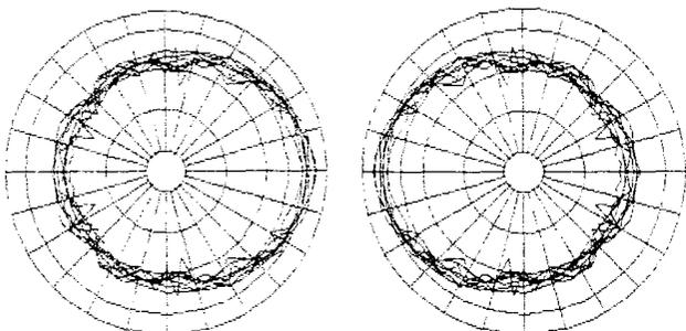
Fig. 8. Measured horizontal radiation pattern for constant-imaging loudspeaker pair. One-third octaves, bundled into octaves 20 Hz to 20 kHz.
