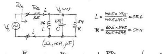
$$Q_{m} = \frac{R}{\omega_{o}L} \qquad Q_{e} = \frac{Re}{\omega_{o}L} \qquad Q_{t} = \frac{1}{\omega_{o}L} \frac{RRe}{R+Re} \qquad \omega_{o} = \frac{1}{\sqrt{LC'}} = 2\pi f_{o}$$
