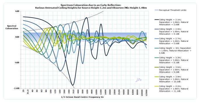
Figure 4: Spectrum Colouration due to a Reflection.
