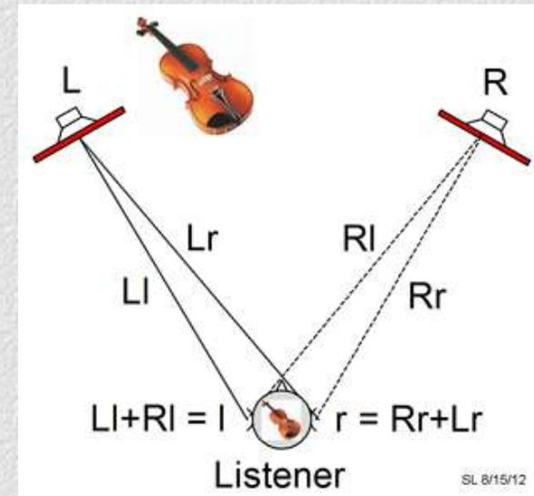
The time differences at the ears determine the phantom **source angle  $\gamma$**
